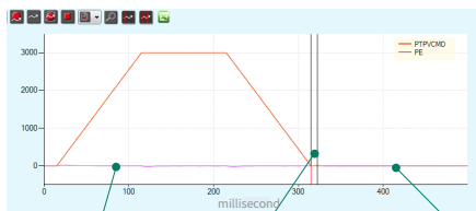
Minimum position error Settling time of almost zero No oscillations at stand-still
