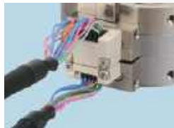
Solder terminals with cables
