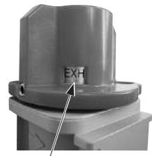
EXH : Air being exhausted
