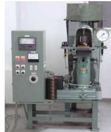
Photo B-14 : SOTA-4-Ball wear test machine
